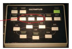
Make sure the slide and coverslip are clean and sealed. Place the slide on the microscope stage. Focus on the sample. Switch between course and fine adjustment using the F/C button.
