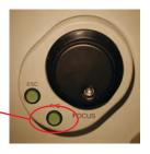
Press the Esc button to move the objective completely away from the sample and press again to bring the objective to the original position.
